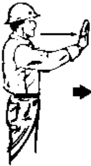
BRIDGE TRAVEL. Arm extended forward, hand open and slightly raised, make pushing motion in direction of travel.
