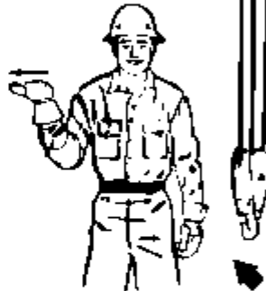
TROLLEY TRAVEL. Palm up, fingers closed, thumb pointing in direction of motion, jerk hand horizontally.
