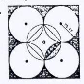
The dotted squares show the maximum area (11,250 sq. ft.) (1,045 m²) that a extinguisher can protect within the limits of the 75-ft. (22.7 m) radius.
