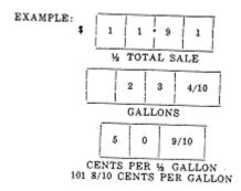
(d) A sign shall be posted at the top of each dispenser that has been set to compute by the price per 1/2 gallon. The sign shall state the following in letters not less than 3/4 of an inch in height and 1/2 inch in width:
